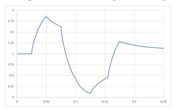
Note that the release stage on both graphs is apparently a bit longer than 60 milliseconds. The specified release time is multiplied internally by a fixed factor to match a commonly-expected release timing.
