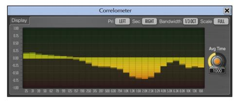
PHA-979's correlation meter works by splitting the incoming signal into bands that are close to ISO frequencies. Band-splitting is performed by means of an array of band-pass filters (the Q factor of the filters depends on the number of bands). This correlation meter can be called an "analog-style" correlation meter.
