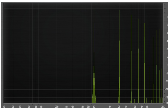
OVC-128 clipping of 1 kHz sine-wave
