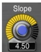
The knob control consists of four parts: the name of parameter it controls, the knob position marker, the center of the knob, and the parameter value readout.
